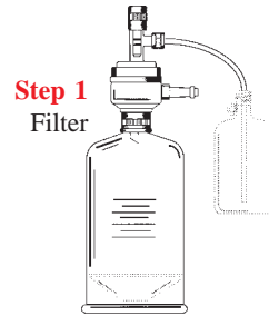
Filter directly into reservoir using the included filtration/degassing cap
