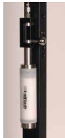
Flash column shown in tower
