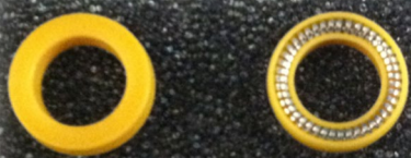
Figure 9, Example of polymer side vs. energizer side of seal.
