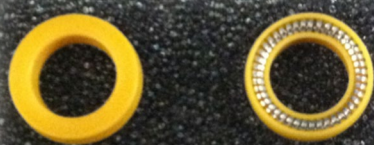
Figure 12, Example of polymer side vs. energizer side of seal.
